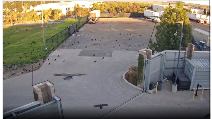
Virtual Barrier analytics ignoring a flock of birds that would have likely caused false alarms on a motion-based algorithm
